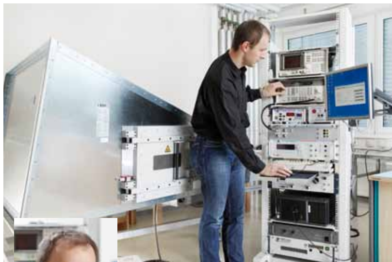
Head of Research and Development, Rudolf Thalbauer, during tests with the new GTEM cell
